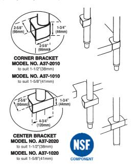
NSF STANDARDS GOVERNING THE USE OF SET SCREWS IN NON-FOOD ZONES REQUIRES THE PLUGGING OF THE HEX SOCKET HOLE AFTER FINAL ASSEMBLY AND TIGHTENING. THIS MAY BE ACCOMPLISHED BY APPLYING A HARDENING TYPE SILICONE SEALANT OR THE USE OF A HOLE PLUG. STANDARD N.S.F. TYPE PUSH-IN PLASTIC HOLE PLUGS ARE AVAILABLE...SPECIFY A10-0020 WHEN ORDERING. SEE PAGE A24.
