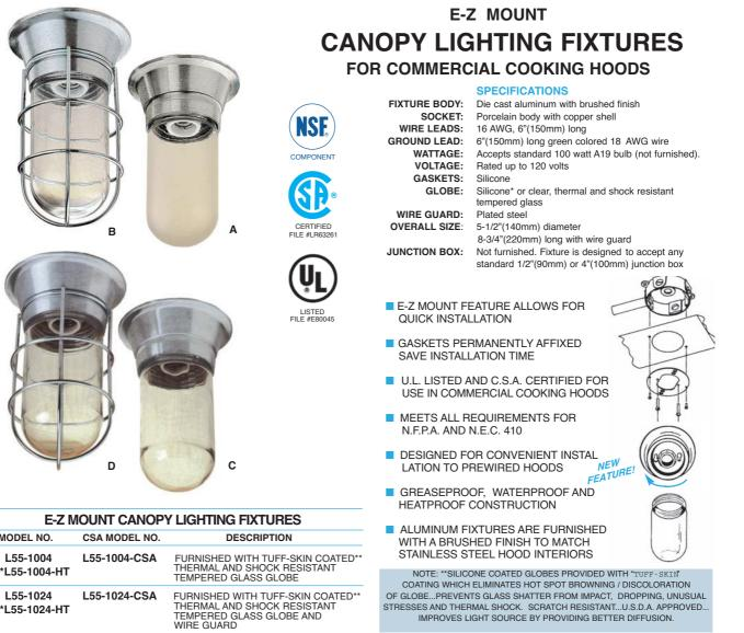
FURNISHED WITH THERMAL, SHOCK С L55-2004 L55-2004-CSA RESISTANT TEMPERED GLASS GLOBE \*L55-2004-HT FURNISHED WITH THERMAL, SHOCK RESISTANT TEMPERED GLASS GLOBE AND WIRE GUARD D L55-2024 L55-2024-CSA \*L55-2004-HT
